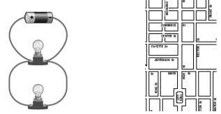
The electrons that flow in this type of circuit can flow through either light, which means they have more energy (volts) to give as they pass, hence a brighter bulb (we divided the resistance between the paths). In a city, if we add more streets, more traffic can flow. So in a circuit, each time we add a pathway, more electrons can flow, creating more current.
