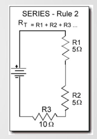
3. The sum of the individual voltage drops equals the total voltage from the power source.
