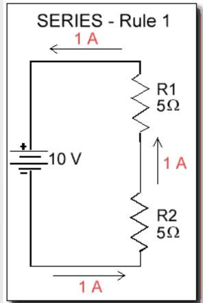
2. The total resistance of a series circuit is equal to the sum of individual resistances.
